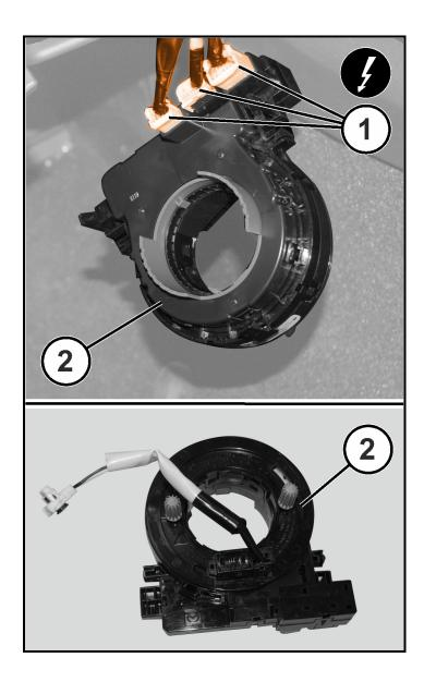
6. Keep the clockspring for airbag module on steering wheel.
